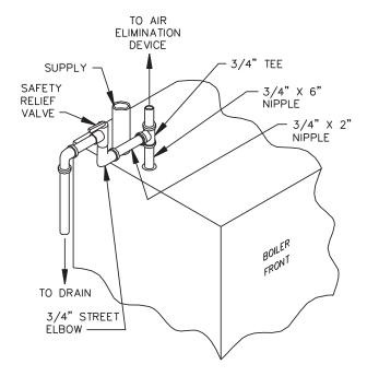
Figure 3: Safety Relief Valve Hook-Up with Air Elimination
