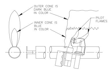
Figure 5: Intermittent Ignition Pilot Configuration and Flames
